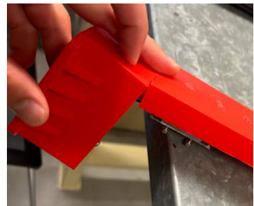
Figure 23 Point of Failure
